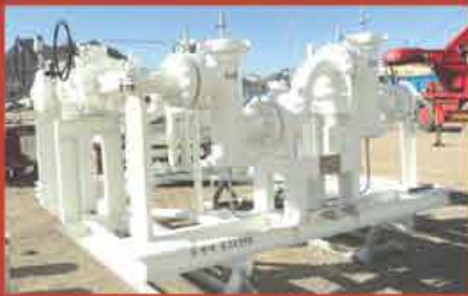
WATER INJECTION FILTER MANIFOLDS
