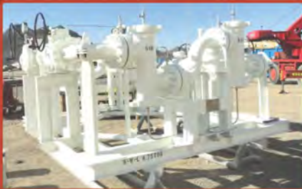
WATER INJECTION FILTER MANIFOLDS
