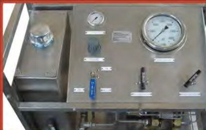
HYDRO TEST PUMP
